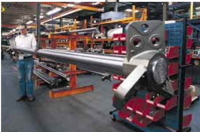
Shafts in excess of 30 feet in length let you specify Series 10 mixers for large tanks without the need for steady bearings.
