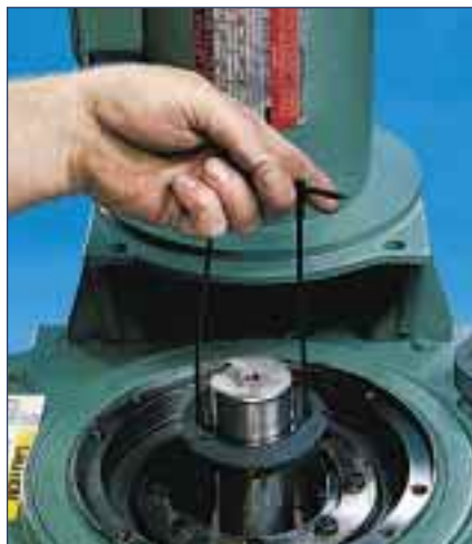
Seal changes are performed in less than 30 minutes. Simply loosen hardware and lower the shaft support collar onto the hub shoulder (1). Once the split coupling has been removed (2), lift off the seal assembly and replace with a new or rebuilt unit (3).
